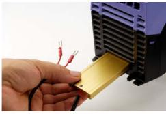
The brake resistor fits into the drive as shown and is secured in place using  $2 \, {}^*$  M4 screws into the rear of the drive.
