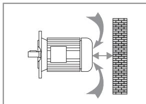
Make sure there is sufficient space between any obstructions and the motor's air intake area to provide adequate cooling for the motor.
