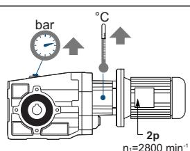
High speed motors, Higher than 1800 rpm, can produce high operating temperatures within the reducer and should only be used for intermittent duty applications. Decrease the reducer's lubricant levels and install a breather plug.
