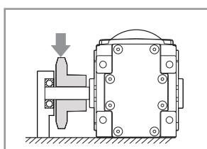
For very heavy radial load, additional output shaft support may be required to prevent premature bearing failure or shaft breakage from bending fatigue.
