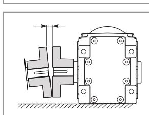
Check shaft and coupling alignment. Check proper coupling gap before to lock all foundation bolts that should be routinely checked.
