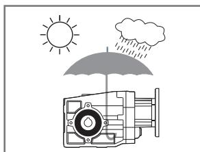
When installed out doors, make sure protection is provided from atmospheric elements.
