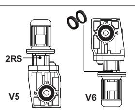
Do not change mounting positions without contacting our factory. Altering the mounting position may require special lubrication provisions which must be installed from the factory. When reducers are mounted in positions V5 or V6 and used in continuous duty applications, replace the upper bearing with a self lubricated style bearing, and we suggest double input seal for V6.
