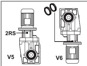
Please specify when ordering if reducer are used in Vertical V5 or V6 mounting position. We normally mount a 2RS self lubricated bearings ( see picture ) for V6 mounting we recommend double oil seals in the input side V6 positions is not recommended for 2 poles motors
