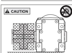
For safety, Buyer or User should provide protective guards over all shaft extensions and any moving apparatus mounted thereon. The User is responsible for checking all applicable safety codes in his area and providing suitable guards. Failure to do so may result in bodily injury and/or damage to equipment.
