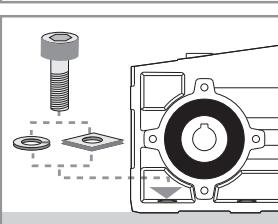
Mount the reducer on a flat surface free of vibration. If high overhung loads are expected, it is advisable to reinforce bolt heads with washers as shown in picture.
