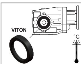
In case of high temperatures we suggest to use FPM (fkm) Oil seals in the output shaft.
