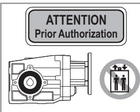
It's compulsory to request HYDRO-MEC authorization to use our gearboxes when the units are used in a man lift or people moving devices.
