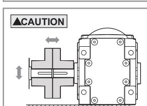
The system of connected rotating parts must be free from critical speed, torsional or other type vibration, no matter how induced. The responsibility for this system analysis lies with the purchaser of the speed reducer.
