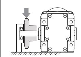
For very heavy radial load, additional output shaft support may be required to prevent premature bearing failure or shaft breakage from bending fatigue.
