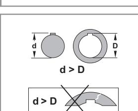
When mounting items to the reducer shaft, appropriate anti-seize and oxidizer compounds should be used, and key dimensions are connected.
