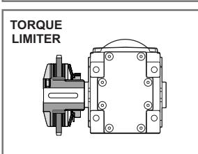
If the application is with high shock loads and sudden stops it's suggested to use mechanical or electronic torque limiting devices.
