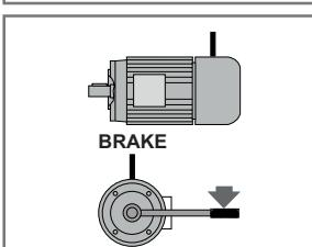
Reducers are not to be considered fail safe or self-locking devices. If these features are required, a properly sized, independent holding device should be used. Reducers should not be used as a brake. Any brakes that are used in conjunction with a reducer must be sized or positioned in such a way so as to not subject the reducer to loads beyond the catalog rating.
